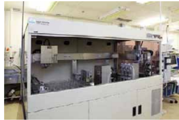
理化学試験用自動前処理装置 Automated pre-treatment equipment for physicochemical tests
