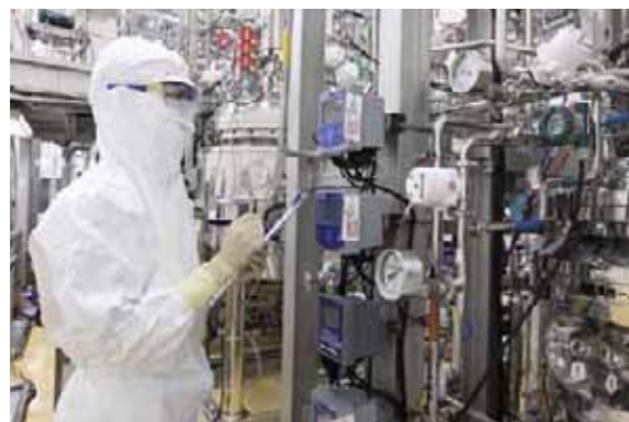
抗体医薬生産のための動物細胞のタンク培養 Tank culture of animal cells for manufacturing antibody drugs
