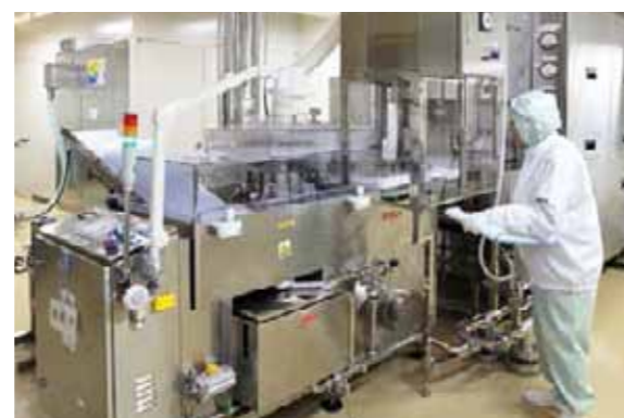
リュープリン注射用(ガラス容器の洗浄乾燥滅菌) Leuprolide acetate for injection (washing, drying, and sterilizing glass cartridges)
