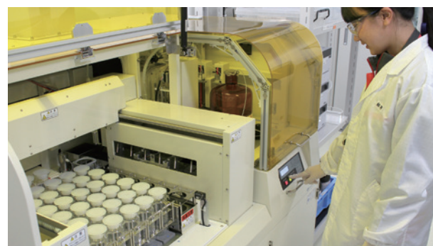
理化学試験用自動前処理装置 Automated pre-treatment equipment for physicochemical tests
